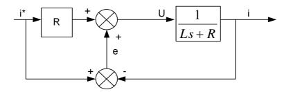
Simulate the system for a unit step and ramp response and crosscheck the results using the final value theorem. Monitor the value of the error and the control signal U.
