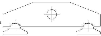
In the diagram of the beam with two feet, a vertical load applied to the beam centre is reacted at the feet. The feet are intended to rotate in their sockets to allow for uneven mounting AND deflection of the beam under load. If the contact regions are specified without allowing tangential movement, a very high load will be on the inner feet corners and the contact regions will be subject to shear loads.
