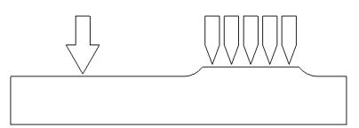
Point Load (or Support) Gives very high stresses: need to ignore or accept local plastic deformation. Load Applied over an Area Need to provide defined area: typically a pad raised 0.1mm. Need to provide large radii to prevent stress concentrations and lots of unwanted elements. Good model of reality.
