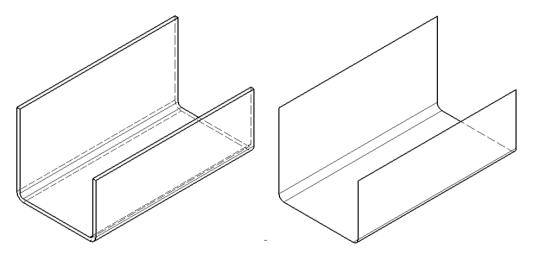
tetrahedral elements but the surface model (IGES) on the right needs only a few plate or shell elements. Whilst the solid model might appear more accurate, the plate / shell model is simpler and will require many fewer approximations.
