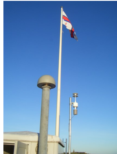
Left: interferogram of 2011 Van earthquake (J Elliott). Right: real-time GNSS station NSLG (P Clarke)
