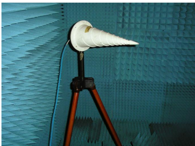
Figure 1 Photographs of the emitting circular polarization antenna (left) and receiving dual-polarization antenna in the anechoic chamber during the initial DP antenna evaluation
