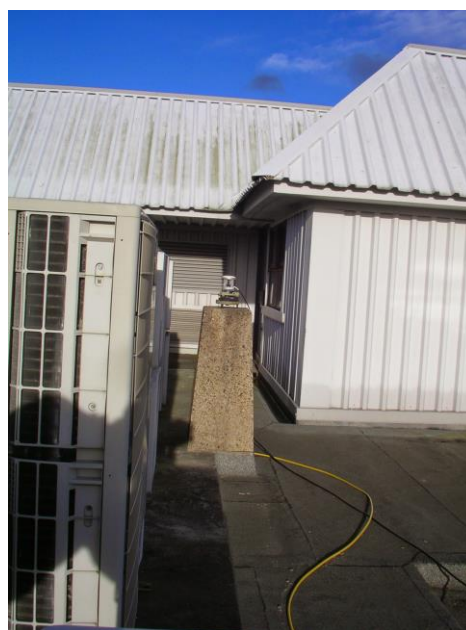
Figure 5 Photos of GPS sites with relatively mild (left) and severe (right) MP conditions. MP is due to NLOS signals reflected/scattered from the flat roof surface below the antenna, parapet walls, the massive metal plate below the antenna (for the mild MP site), air conditioning units and metal walls and roof of the bulkhead construction (for the severe MP site)
