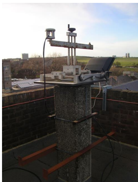
Figure 5 Photos of GPS sites with relatively mild (left) and severe (right) MP conditions. MP is due to NLOS signals reflected/scattered from the flat roof surface below the antenna, parapet walls, the massive metal plate below the antenna (for the mild MP site), air conditioning units and metal walls and roof of the bulkhead construction (for the severe MP site)
