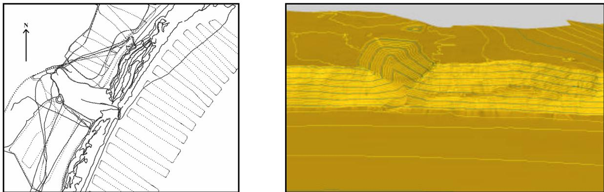
Figure 1. Plan View (Left), and 3D View (Right) of GPS DEM Created for Filey Country Park, 2001 Survey
