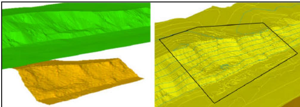
Figure 3. Unmatched Surfaces at Southern End of Strip (Left), Showing Photogrammetric DEM Below GPS DEM, and (Right) Merged Surface (1m Contours)
