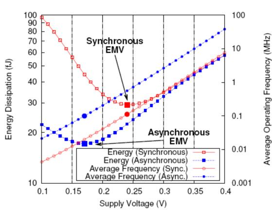
Asynchronous (selftimed) logic can provide completion detection and thus reduce the interval of leakage to minimum, thereby doing nothing well!
