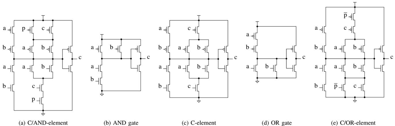
Figure 5: Transistor-level implementations of specialised and parametrised gates
