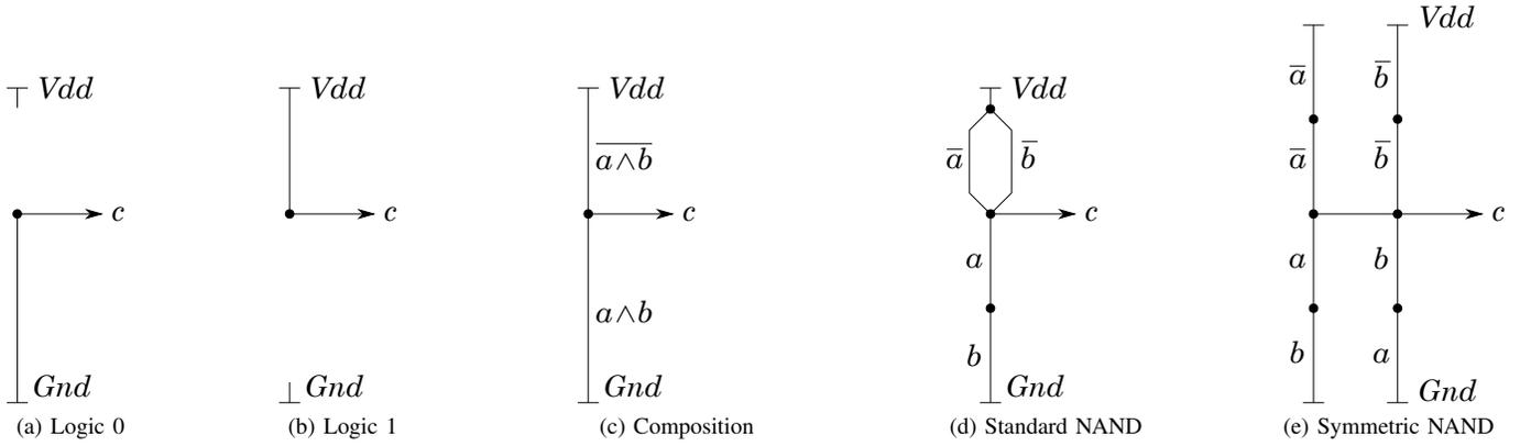
Figure 4: NAND gate synthesis stages
