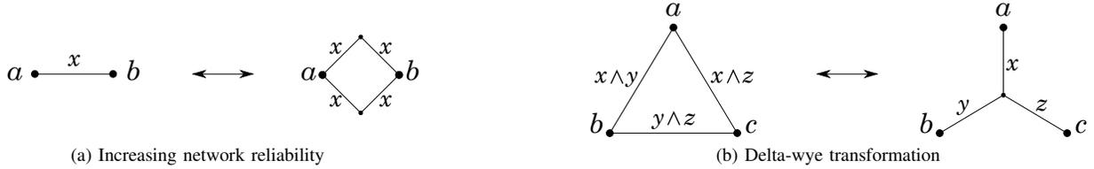
Figure 2: Examples of functionally equivalent transformations
