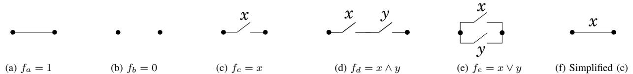
Figure 1: Switching networks and their connectivity functions
