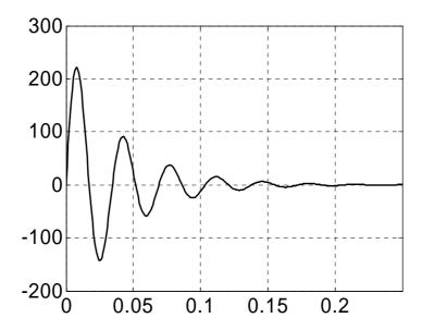
This is happening because the electrical time constant (L/R=0.0192) is much smaller (i.e. faster) than the mechanical one (i.e. J/B=50000).
