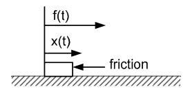
$$\Sigma F = ma \Leftrightarrow f - f_{friction} = ma \Leftrightarrow f - B\omega = ma \Leftrightarrow f - B\frac{dx}{dt} = m\frac{d^2x}{dt^2}$$
