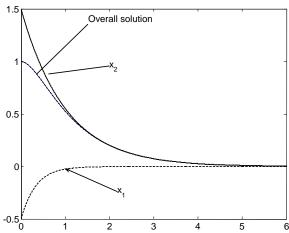
• Roots are real and equal:  $r_1=r_2$  ( $A^2=4B$  Critically damped system)
