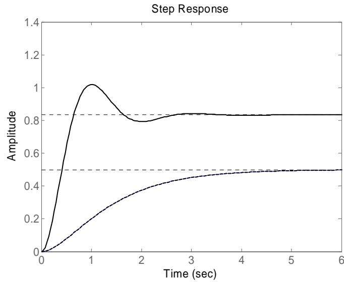
So apart from faster system and smaller steady state error we have oscillations!
