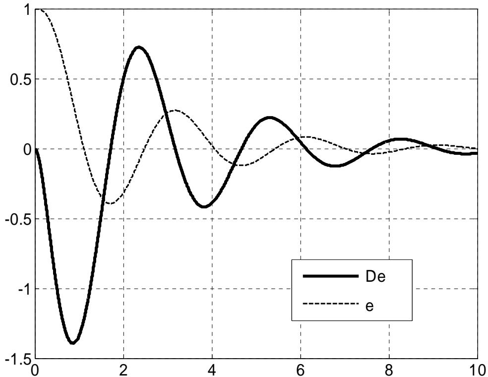
Maximum value of De just before e=0. So De can control the oscillations:
