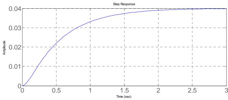
c.  $\omega_n = 0.5 \text{ rad/s}$ ,  $\omega_n = 5 \text{ rad/s}$ ,  $\omega_n = 50 \text{ rad/s}$  (keep  $\zeta = 0.5, k = 1$ )
