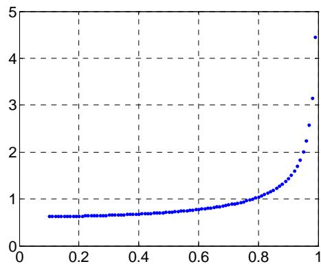
14. Using the specific formula plot the peak time versus the natural frequency for  $z=0.1\text{rad/s}$ .
