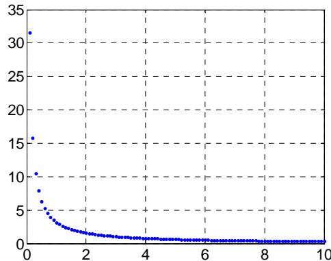
15. Using the specific formula plot the settling time (5% and 2% in the same graph) versus the natural frequency for  $z=0.1\text{rad/s}$ :
