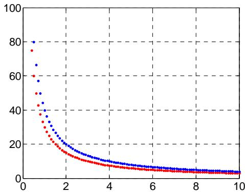
16. Using the specific formula plot the settling time (5% and 2% in the same graph) versus the damping factor for  $\omega_n=5\text{rad/s}$ :
