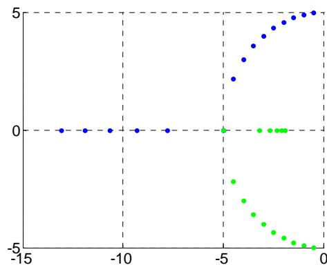
8. Assume a system with  $\zeta = 0.5$  and  $\omega_n = 5\text{rad/s}$ . Use an m-file to calculate and hence plot the pole location in the s-plane for  $k \in [0.1, 2]$  (use a step size of 0.5).
