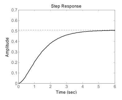
It is clear that the addition of the two zeros near the two complex poles made the system overdamped and hence verified the statement that the response of the system depends on poles that are close to the jw axis and they are isolated (i.e. far away from zeros).
