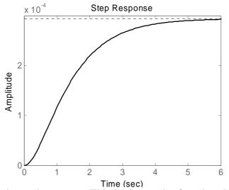
Time (sec) The system has an overdamped response. This is due to the fact that the two real poles are far closer to the jw axis than the two complex poles. Therefore the dominant poles are the two real poles and the overall behaviour of the system is MOSTLY influenced by these two real poles.
