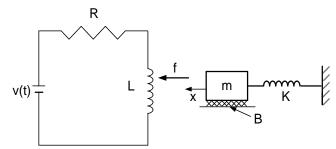
The force of the magnetic field is directly related to the current in the *RL* network. The force that is exerted on the object is  $f = k_A \frac{i^2}{x^2}$ , where  $k_A$  is a
