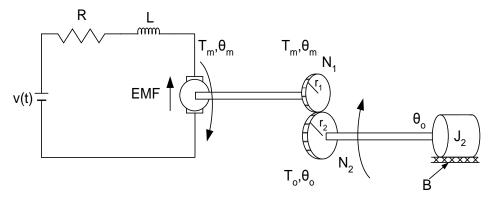
The shaft of the separately excited DC motor is connected to the load  $J_2$  through a gear box.
