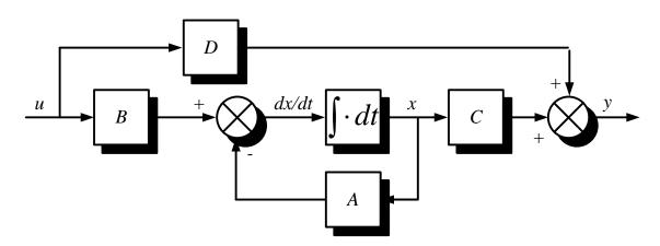
The state of a system is a complete summary of the system at a particular point in time. If the current state of the system and the future input signals are known then it is possible to define the future states and outputs of the system.
