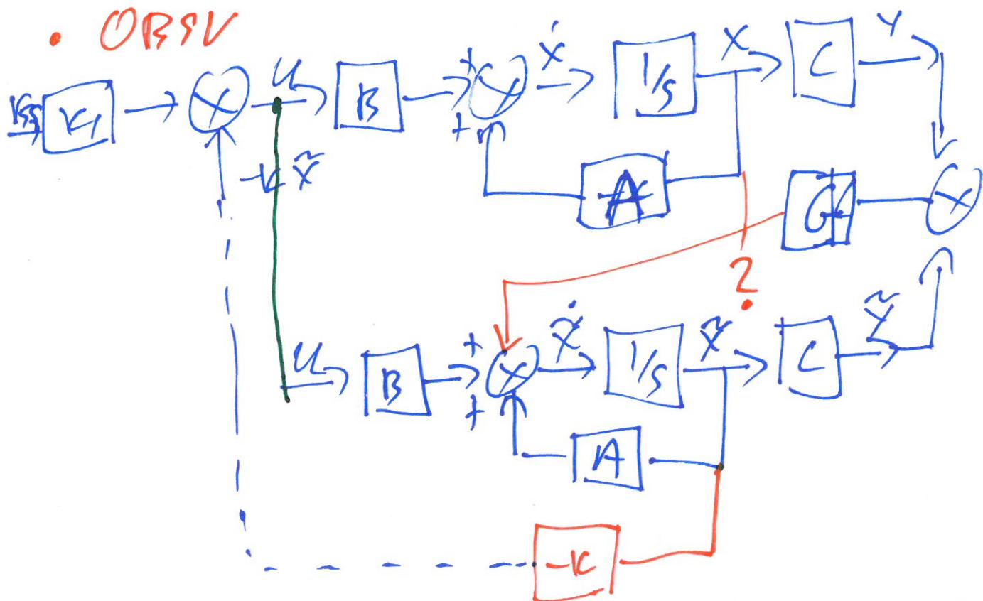
$$G = ? \quad \text{pole placement} \quad \dot{e} = (A - Gc)e$$
