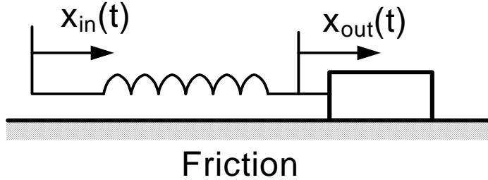
$$K(x_{in} - x_{out}) - B \frac{dx_{out}}{dt} = m \frac{d^2 x_{out}}{dt^2} \xrightarrow[IC=0]{LT}$$
