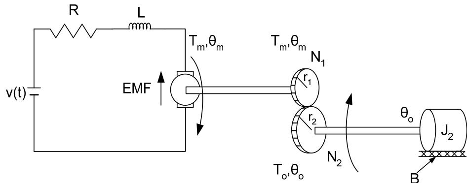
$$\left. \begin{aligned} J \ddot{\theta}_0 &= T_0 - B \dot{\theta}_0 \\ T_0 &= \frac{n_2}{n_1} T_m \\ T_m &= K_T \varphi i_a \end{aligned} \right\} \Rightarrow J \ddot{\theta}_0 = \frac{n_2}{n_1} K_T \varphi i_a - B \dot{\theta}_0 \Rightarrow$$
