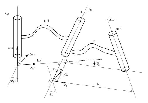
$^{n-1}T_n = Rot(x, a_{n-1})Trans(l_{n-1}, 0, 0)Rot(z, \theta_n)Trans(0, 0, d_n) \text{ and } {}^{R}T_H = {}^{0}T_1 {}^{1}T_2 {}^{2}T_3 \cdots {}^{n-1}T_H$
