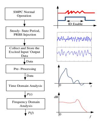
Fig. 3. Non-parametric identification procedure of SMPC.
