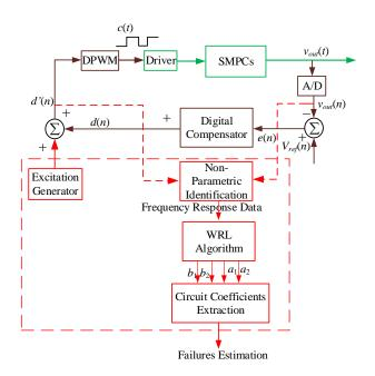
Fig. 17. Dual estimation scheme based on WLS algorithm.
