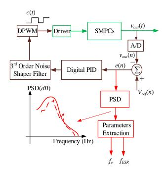
Fig. 15. PSD estimation block diagram.
