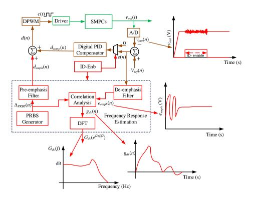
Fig. 13. Non-parametric correlation block diagram.
