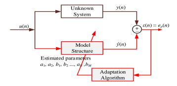
Fig. 6. General block diagram of parametric identification.
