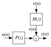
Fig. 4. General linear model transfer function.
