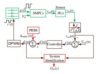
Fig. 2. Closed loop system identification for SMPCs.
