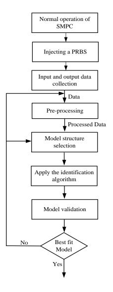
Fig. 5. Parametric identification procedure of SMPC.
