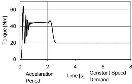
Fig. 10 Torque response for test 1
