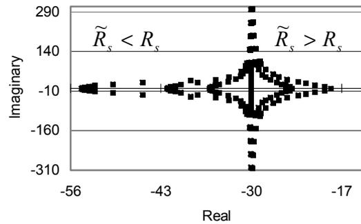
Fig. 6 Root locus for stator currents
