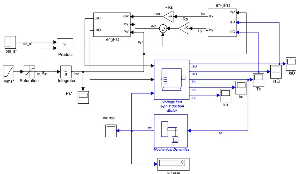
Fig. 7 Simulink model for the Open loop control scheme
