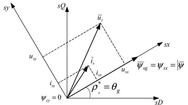
Fig. 2 Stator flux orientation
