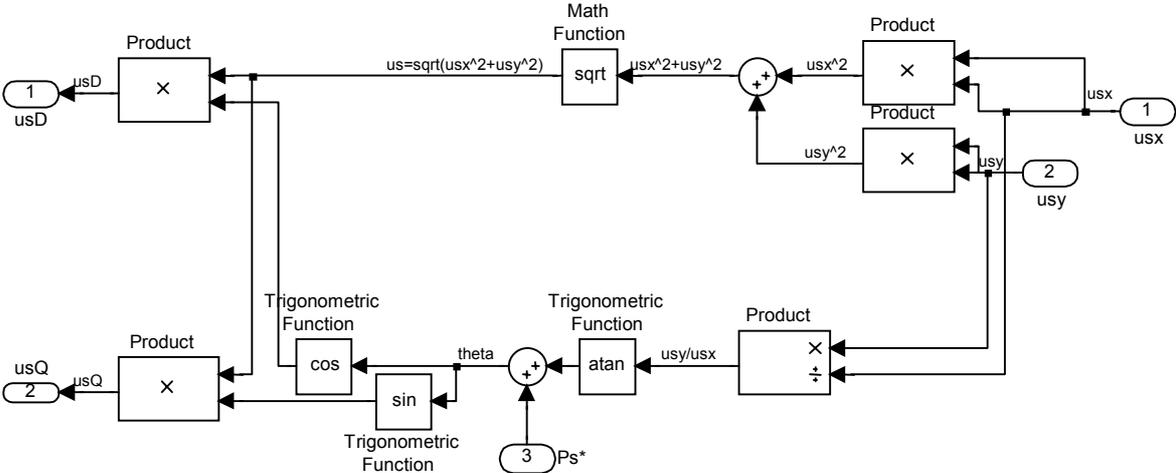
Fig. 8 Sub-block: calculates usD and usQ from usx and usy
