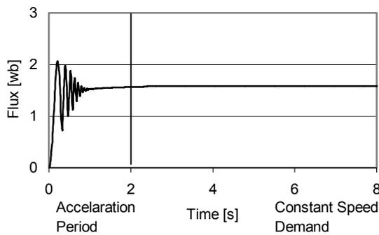
Fig. 14 Stator flux linkage response for test 1
