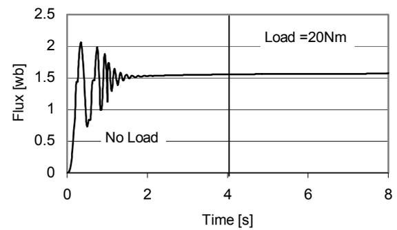
Fig. 15 Stator flux linkage response for test 2
