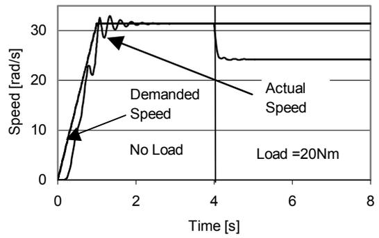
Fig. 13 Speed response for test 2
