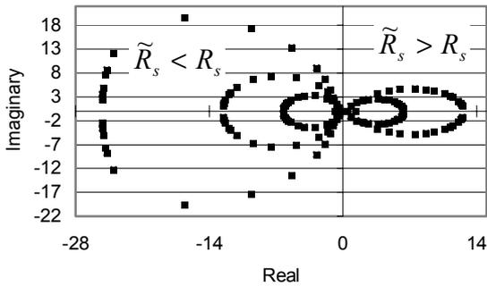
Fig. 5 Root locus for stator fluxes
