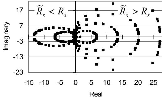
Fig. 4 Root locus for stator fluxes
