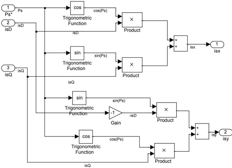
Fig. 9 Sub-block: calculates isx and isy from isD and isQ
