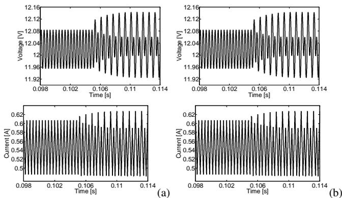
Fig. 5. System output voltage and current time responses showing a loss of period-1 stability at  $time = 0.105s$  caused by an increase of input voltage from 24V to 25V (a) original model (b) TS fuzzy model.
