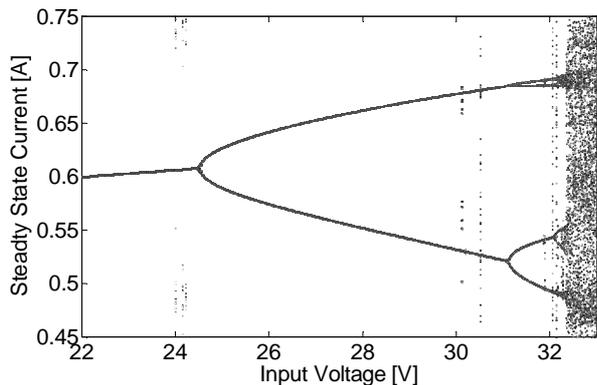
Fig. 6. Bifurcation diagram of the TS fuzzy model of the buck converter with the input voltage as the bifurcation parameter.
