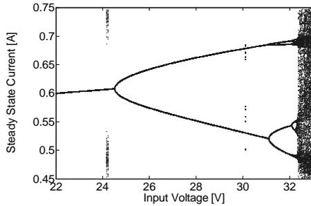
Fig. 4. Bifurcation diagram of the buck converter with the input voltage as the bifurcation parameter.
