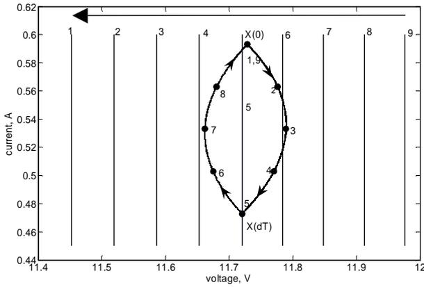
Fig. 3. Period-1 limit cycle indicating the location of the time varying switching surface.
