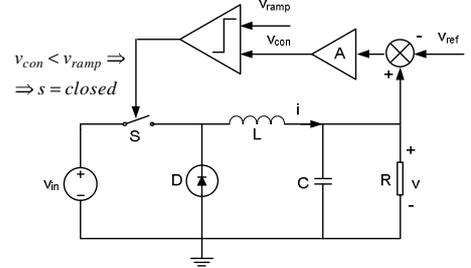
Fig. 1. Voltage mode controlled buck dc-dc converter.
