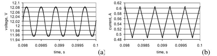
Fig. 2. Nominal period-1 operation of the buck converter: (a) output voltage, (b) output current; fixed parameter values  $V_{in} = 24V$ ,  $V_{ref} = 11.3V$ ,  $L = 20mH$ ,  $R = 22\Omega$ ,  $C = 47\mu F$ ,  $A = 8.4$ ,  $T = 1/2500s$  and the ramp signal varies from 3.8V to 8.2V.
