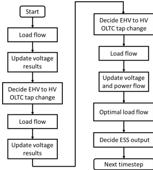
Figure 1 Flow chart of the control scheme
