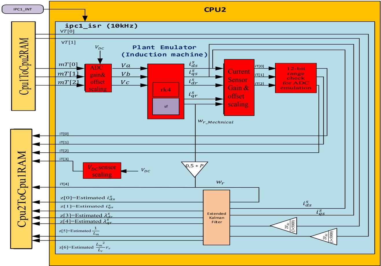
Fig.2. Implementation of extended Kalman-filter and induction motor emulator in F28377d
