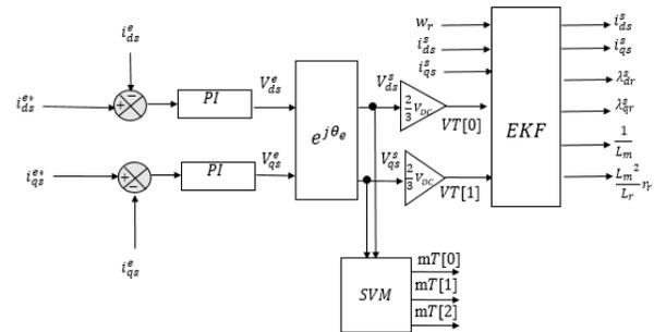
Fig. 1. Imputes and outputs of proposed augmented states for EXF
