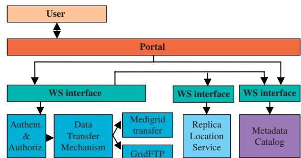
Fig. 2. High-level architecture of MEDIGRID data services layer (WS = web service).
