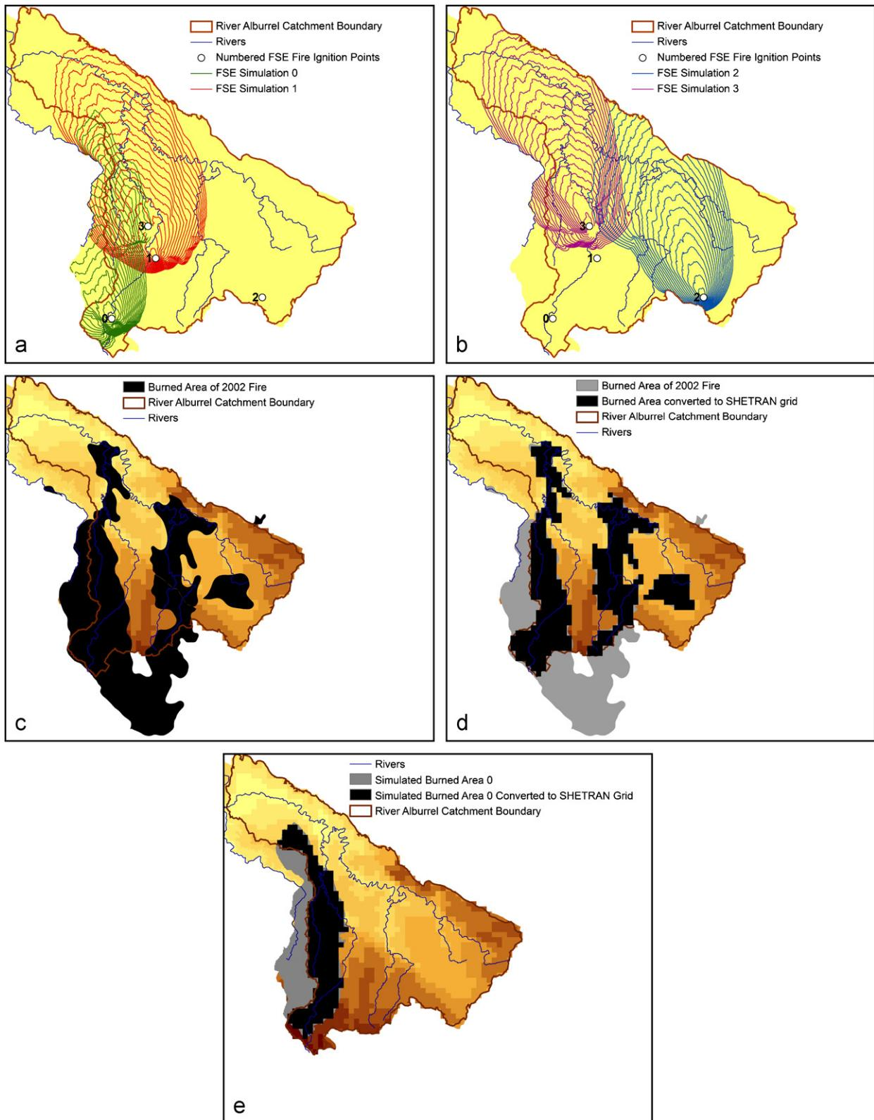
Fig. 7. Four FSE simulation outputs for fires with various origins (a) simulations labelled 0 and 1, and (b) simulations labelled 2 and 3. All simulations ran for 20 model hours. (c) Real extent of 2002 fire, and (d) transformed into SHETRAN input grid. (e) SHETRAN input grid based on FSE simulation labelled 0.
