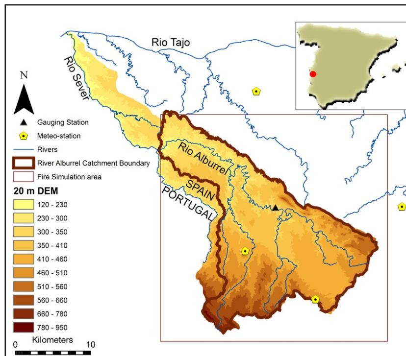
Fig. 5. Location and Digital Elevation Model (DEM) ( $20 \times 20$  m grid) of the study area. FSE is applied to boxed area right of Sever River (shown by DEM), whilst SHETRAN is applied to River Alburrel catchment only. Positions of rivers longer than 10 km, one river gauging station and four rain gauges are also shown.
