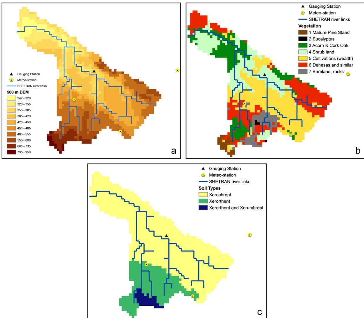
Fig. 6. (a) SHETRAN 500 m DEM grid showing river network, (b) vegetation categories and (c) soil types.
