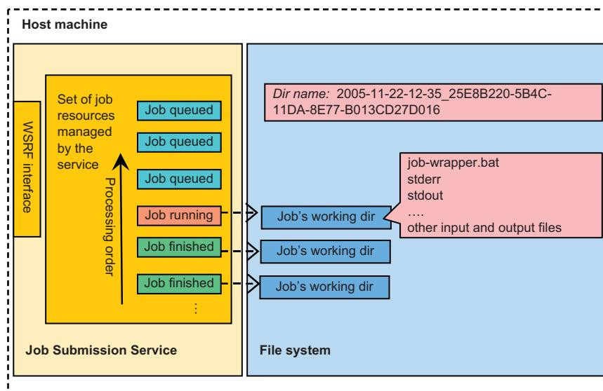
Fig. 4. Schematic of job submission service and its associated resources on a host machine.
