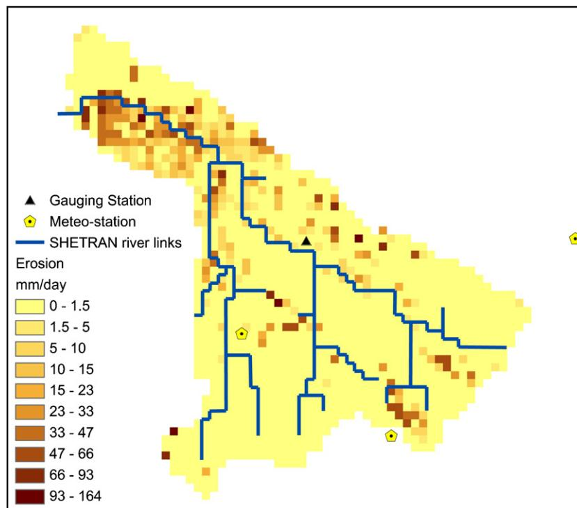
Fig. 8. Example of soil erosion rates over catchment for day 179 of SHETRAN simulation (mm/day).
