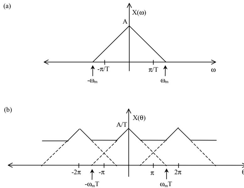
Figure 8.2: Sampling of a band limited signal below the Nyquist rate: (a) Fourier transform of the continuous-time signal; (b) Fourier transform of the sampled signal.
