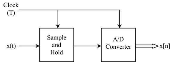
Figure 8.4: Schematic diagram of sampling by an A/D converter.
