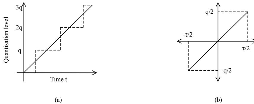
Figure 8.5: (a) Quantisation of the input signal. (b) Quantisation error.
