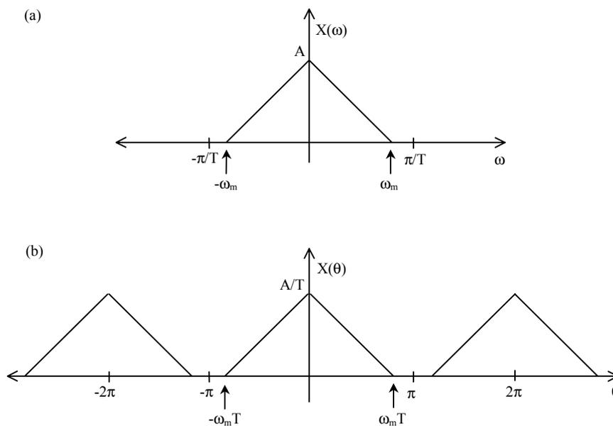
Figure 8.1: Sampling of a band limited signal above the Nyquist rate: (a) Fourier transform of the continuous-time signal; (b) Fourier transform of the sampled signal.
