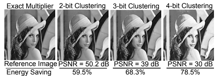
Figure 8: Output quality after applying Gaussian blur filtering to three different versions of the proposed (8 \times 8) multiplier.
